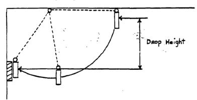
Drop height is determined from center line of action at rest against impact area
