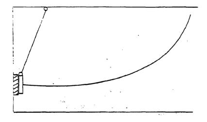
Adjust firearm placement so that gun is parallel and square to the impact area. Gun is to be leveled in each position prior to drop.
