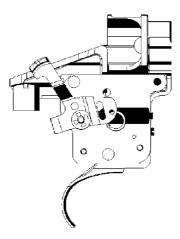
The dark blue part is the translating trigger block that moves back and forth with the operation of the safety arm. There is an adjustment screw that sets allowable trigger motion on safe to a minimum level.
