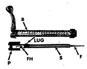
The total number of components in this sub-assembly is twelve. The bolt handle, body, and head are made as one piece. The firing pin head is pinned to the firing pin and retains the bolt plug and firing pin spring. The firing pin subassembly is assembled to the bolt by a "Bayonet" type lug system. This is done by pushing the firing pin assembly into the bolt and rotating the entire assembly. (See Photo #2)
