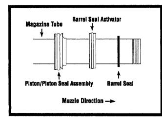
A barrel seal activator is used on the Model 11-87 12-gauge Super Magnum shotgun to improve performance when using light 2<sup>3</sup>/4" loads. Refer to the diagram (left) for the proper position of the piston/piston seal assembly, barrel seal activator and barrel seal. Removal of the barrel seal activator is recommended when using 3" or 3<sup>1</sup>/2" loads.
