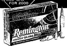
The outstanding velocity and energy performance of our new Ultra Mag<sup>TM</sup> cartridges comes from their innovative case design that dramatically increases powder capacity. The increased volume comes from headspacing on the shoulder of the case rather than a belt. The result is a non-belted magnum, with a larger case diameter. Two more benefits of a non-belted case are improved accuracy and longer case life.
