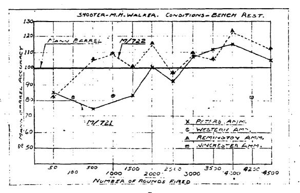
It will be noted from the above that as the mean radius of the test gun decreases below that of the Mann barrel, a better than 100% accuracy is obtained. This indicates the assumption that Mann barrel yields optimum accuracy is in error. It is unimportant, however, since a measure of change in accuracy was desired and such a measure is obtained by this method.
