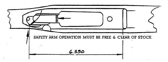
Reinforcing screw bent forward .050" Max.
