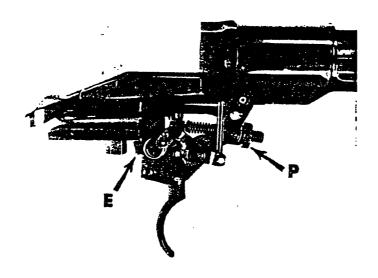
Browning explains how to adjust trigger pull in their owner's manual but does not mention anything about the engagement adjustment. The fire control assembly is screwed and pinned to the receiver and has openings on either side that allows access to the sear/trigger engagement. The sear and trigger engage directly in this fire control.
