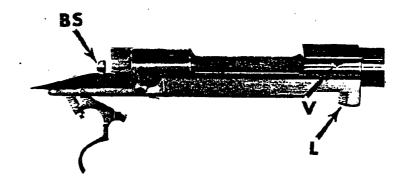
The bolt stop button protrudes up through a small cut in the left side of the receiver tang. (Photo #1) This must be pressed down to remove the bolt, but does not have to be touched when the bolt is inserted back in. However, the bolt does slide in much easier when this button is depressed.
