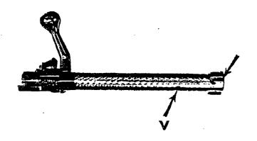
A plunger type springed ejector is mounted in the bolt face. The extractor is a claw type that is plunger actuated. It slides in a "T" cut in the right locking lug. (Photo #5)
