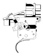
The dark blue part is the translating trigger block that moves back and forth with the operation of the safety arm. There is an adjustment screw that sets allowable trigger motion on safe to a minimum level.
