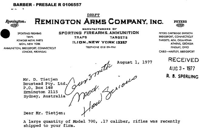
It has come to our attention that a very minor operation has not been properly performed on the bolt face. The firing pin hole in the bolt face requires a slight radius to prevent the possibility of a primer blanking out in the .17 caliber rifle upon firing. This is the only caliber in our entire line of rifles requiring a radius of the firing pin hole.
