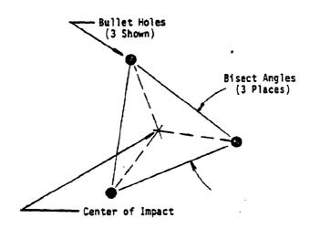
The center of impact may also be found relative to the point of aim be measuring the horizontal and vertical distance of each bullet hole from the point of aim and averaging.
