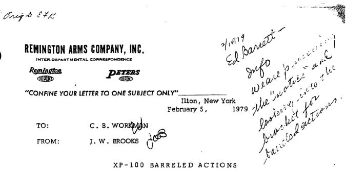
We now sell barreled actions from our Custom Repair Department in Ilion. We sell the barreled action minus the trigger balance. The XP-100 does not have an adjustable trigger for pounds pull. The sear block spring and the trigger balance spring must both be overcome to release the sear from the sear block.
