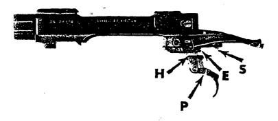
The sear in this rifle is pinned to the receiver while the trigger is attached to the fire control housing. (See Photo #8) The trigger and sear engage directly here.
