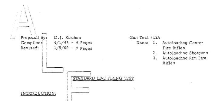
This test is performed for the same reasons as Test #12. It differs from Test #12 in that it covers autoloading firearms. The functional characteristics of which differ considerably from manual action firearms.
