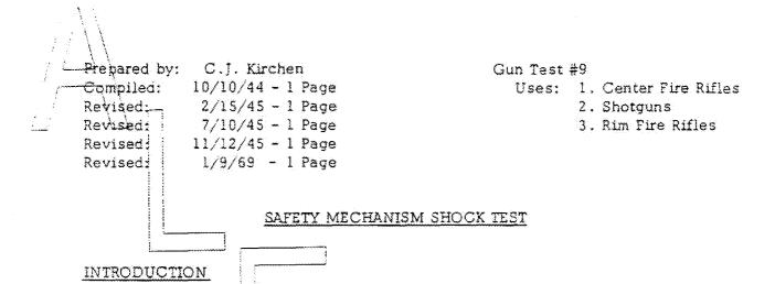
A common source of accidents with firearms is accidental discharge. A safety mechanism is provided to insure against accidental discharge. This test is intended to determine how much shock, if any, will cause the safety mechanism to fail to function properly and allow the gun to be discharged.
