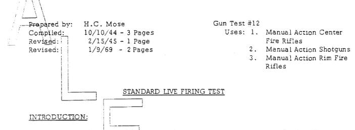
Live ammunition is fired in guns under test to observe the function of both the gun and ammunition and to evaluate certain characteristics of the gun. The characteristics of components, new or unused in design, material, method of production, heat treatment and assembly procedures are obviously pertinent.
