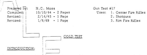
This test is performed with live ammunition for the purpose of determining the gun's functional characteristics at low temperatures. A temperature of  $-20^{\circ}$ F is possible with existing equipment and this temperature appears satisfactory for this test. It is felt that this temperature approaches conditions encountered in actual service.
