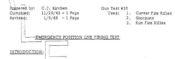
This test is performed for the same reasons as Test #12 and #12A. It differs in that firing is done with the gun in other than normal position. While these positions may be considered extreme, it is desired to know whether mere position is an important factor in gun operation.
