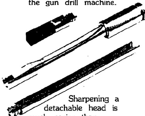
Sharpening a detachable head is much easier than sharpening a long drill of one piece construction.
