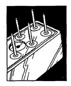
Dissimilar metals, carbon steel, Kovar, copper, tungsten, tantalum, stainless steel, etc. No flux or filler material required. Virtually no distortion of surrounding materials. Ideal for seam and high speed spot welding.
