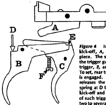
Figure 4 In this double set trigger, the kick-off, A, replaces the usual trigger piece. The set mechanism, mounted in the trigger guard, includes a rear setting trigger, B, and a front firing trigger, C. To set, rear trigger is pulled until ledge E is engaged. A pull on the firing trigger releases the set rear trigger, which a spring at D throws upward to strike the kick-off and thus fire the rifle. The pull of such triggers varies from an ounce or two to several pounds.
