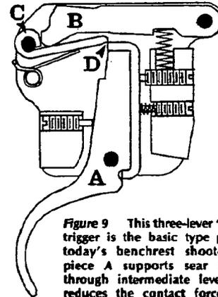
Figure 9 This three-lever "two-ounce" trigger is the basic type preferred by today's benchrest shooters. Trigger piece A supports sear B indirectly through intermediate lever C, which reduces the contact force at release point D enough to make pull as light as two ounces possible. This Remington trigger is fully adjustable also.
