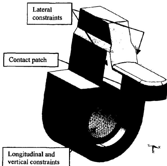
Figure 3. Constraints placed on model.
