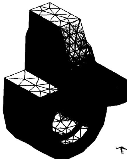
Figure 2. Meshed model of firing pin head.
