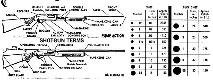
**GAUGES**—Shotguns are made in several well-known gauges, 12, 16, 20, 28 and 410. Other gauges have been made in the past but are not at present in common use. These include 4, 8, 10, 14, 24 and 32 gauges.
