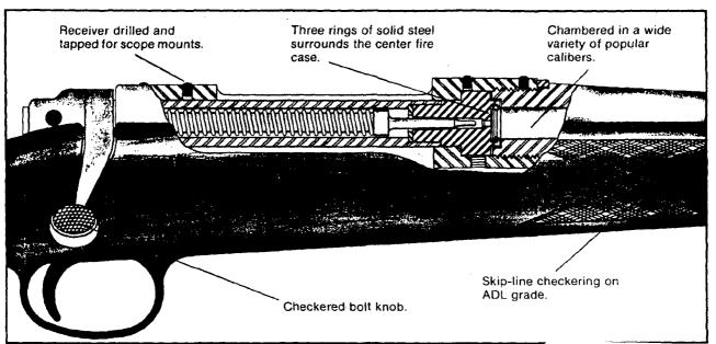
calibers...it is America's best selling bolt action center fire rifle. In big game hunting, dependable performance is of primary importance. The 700's antibind bolt and stainless steel magazine follower assure smooth operation without bind or drag. The action is one of the strongest ever designed. Bolt face, barrel and re-
