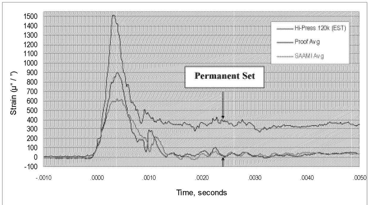
Figure 11: Strain Data for Abusive testing of gun A9.
