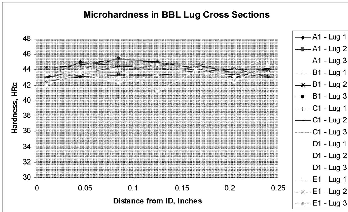
Figure 7: Locking Lug Microhardness Data.
