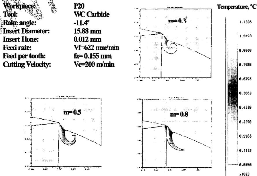
Figure 4: Influence of Friction Factor m on Chip Formation and Temperatures
