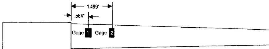
Chamber Strain Test with Heat Treated Barrels- M/710 Magnum Bolt Action Rifle
