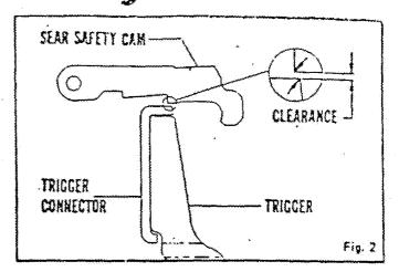
Sear safety cam and trioper connector engagement of .015" – .020" on field rifles and .010" – .015" on target rifles is critical (see Fig. 3). Replace any worn or damaged parts. To adjust, close bolt and place safety OFF SAFE. Turn trigger engagement screw clockwise until rifle fires. Turn screw counterclockwise % turn (90°) and check engagement, Isee note A). Corners must be sharp. (Arrows).
