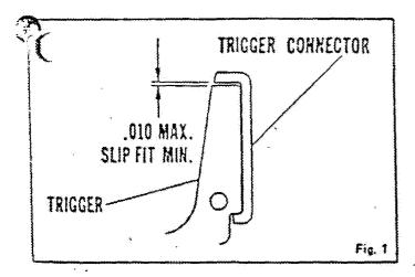
When replacing trigger housing assembly, take care not to pend or spring the housing. Sear safety cam should pivot freely. To check, remove bolt, move safety to OFF SAFE, pull trigger and press down on rear of sear safety cam and release.
