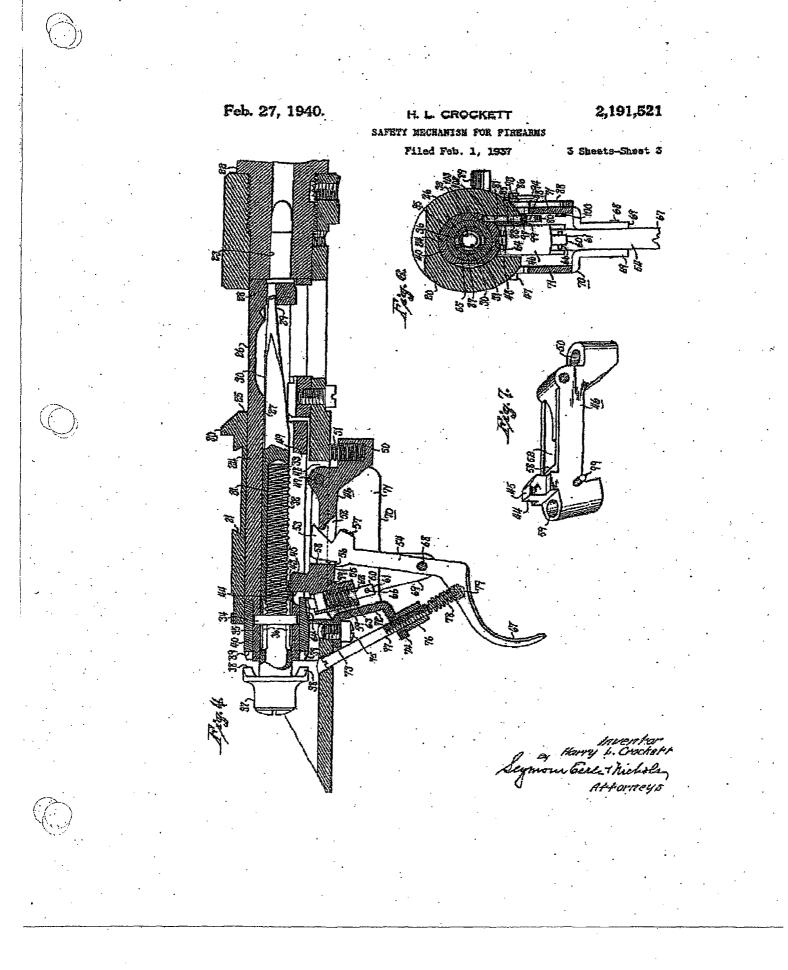
standing from a pivotal sear 46. The said sear is pivotally mounted adjacent its forward end by means of a transverse pivot-screw 41, in a vertically-extending passage 48 formed in the under side of the receiver 20. The said scar-nose 45 of the sear 48 projects upwardly for the engagement of its rear face 44 with the cocking-shouldsr 43, through a longitudinal clearance-slot 49 formed in the under side of the bolt 26.
